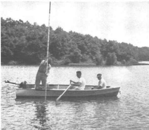
Measuring amount of sediment at the bottom of a water-supply reservoir
