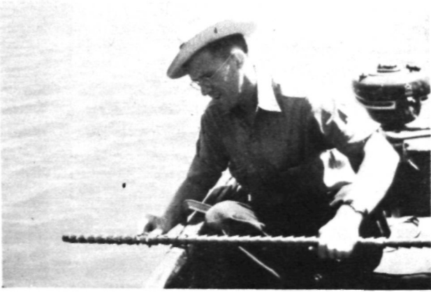
FIG. 4. USE OF THE SPUD IN MEASURING SEDIMENT THICKNESS.
