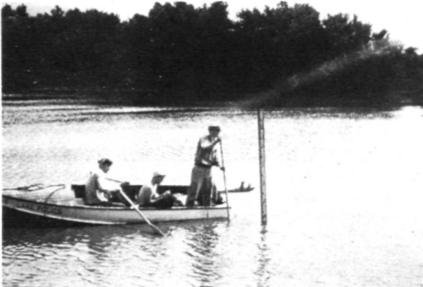
FIG. 5. USE OF THE SOUNDING POLE IN MEASURING SEDIMENT THICKNESS.
